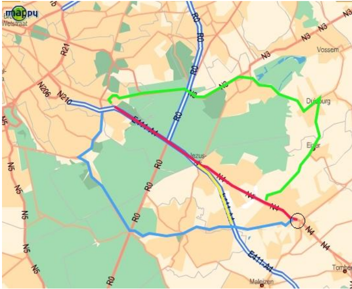
Fig. 5. A car at the circle (at the bottom right) has three possible routes: straight ahead, left, and straight on and then right. In the current situation, the car follows the route straight ahead, which has the minimal cost.
